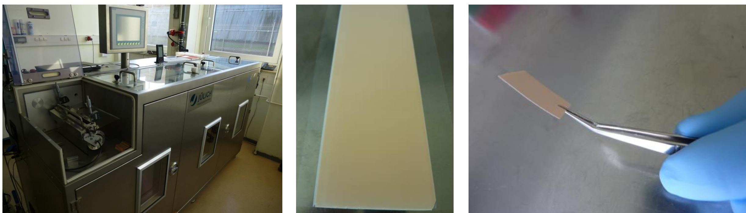
Fig.3: (l.) A tape casting line at IEK-1 can be used for large scale tape casting. (m.) Al-LLZ tapes were successfully processed by tape casting with a gap size of 250 \mu\text{m} and 500 \mu\text{m} . (n.) Solid electrolytes with a green tape thickness of 90 \mu\text{m} and 180 \mu\text{m} were used for further sintering studies.
